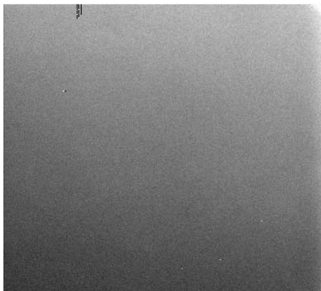
FIG. 6.—Image formed by the division of a flat field taken with the diffuser in place by a flat field taken without the diffuser in place. This test was done with separate flat fields from those used previously.
